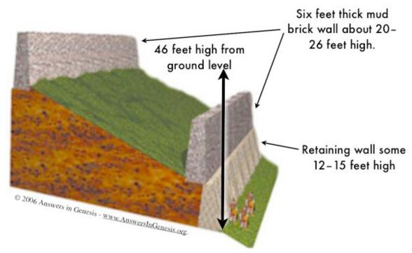
The city of Jericho was built on a hill, surrounded by a great earthen rampart, or embankment, with a stone retaining wall at its base. The retaining wall was some 12-15 ft high. On top of that was a mudbrick wall 6ft thick and about 20-26 ft high (Sellin and Watzinger 1973)
